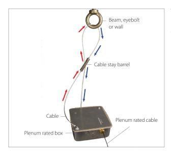
Wrap the cable around a beam, eyebolt or hanger. Next, slip the cable through the top of cable stay barrel pulling excess cable until taut.
