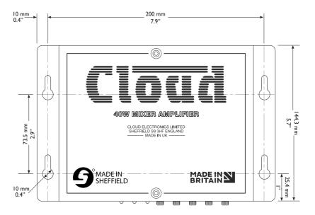
If using the MA40 in a free-standing situation, the self-adhesive feet (supplied with the amplifier) should be fitted. The amplifier should always be stood on a flat surface. Care should be exercised in selecting a location for a free-standing unit, which should allow ventilation but be clear of any liquid or similar hazard.
