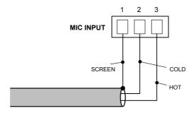
The MA40's microphone pre-amplifier is an electronically balanced, transformer-less design configured for optimum low noise performance. The input impedance is greater than 2 kohms and is suitable for microphones in the 200 ohm to 600 ohm range. The microphone signal path includes a fixed high-pass filter. This attenuates the response below 120 Hz, which helps to reduce the effects of microphone handling noise.
