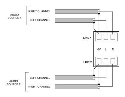
The two line inputs are summed together internally, though Line input I can be configured to have priority over Line input 2, see "Line I Priority" on page 18.
