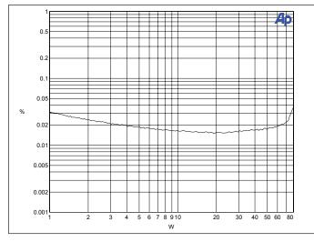
THD+N (%) vs Output Power (W) into a 40hm load. 1kHz sine wave input
