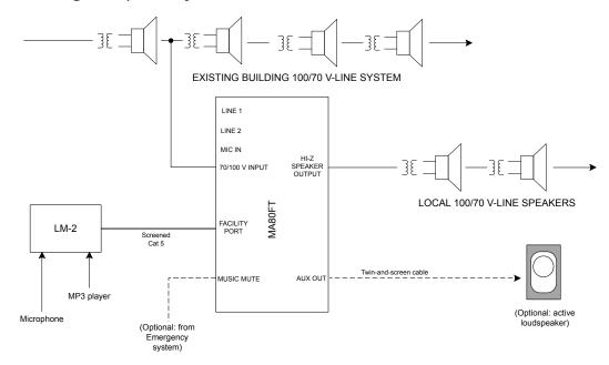
In this example, an MA80FT is used to provide local music and microphone amplification in a particular part of a building (possibly a new extension), while at the same time ensuring that the local loudspeakers are integrated with the main building PA/VA system.
