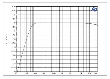
Frequency Response of Line input in both Low & High Impedance output. Low Z output: 4ohm load High Z output: 1250hm load (65 Hz HPF evident
