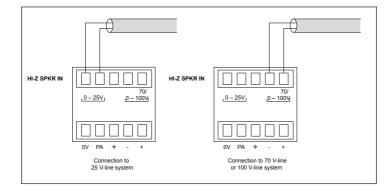
Note that the 70/100 V input is suitable for use with either 70 V-line or 100 V-line systems.
