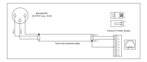
An unbalanced source may also be connected; the use of a balancing transformer is recommended.
