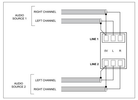
Unless a Cloud remote control plate or module such as the RSL-6 or LM-2 is in use, the two line inputs are summed together internally, though Line input 1 can be configured to have priority over Line input 2, see "Hi-Z input" on page 24.
