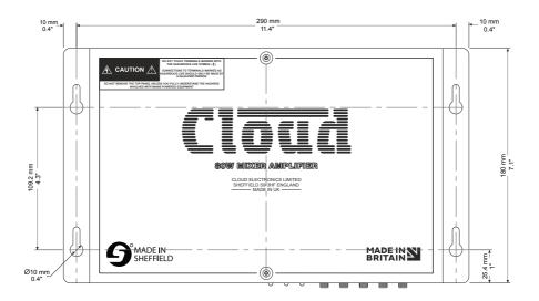
If using the MA80FT in a free-standing situation, the self-adhesive feet (supplied with each amplifier) should be fitted. The amplifier should always be stood on a flat surface. Care should be exercised in selecting a location for a free-standing unit, which should allow ventilation but be clear of any liquid or similar hazard.
