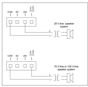
When driving 25/70/100V-line loudspeaker systems there is a risk of transformer core saturation at high levels and low frequencies, which can produce distortion. To prevent this, the MA80FT's output stage is provided with a 65 Hz high-pass filter, which is automatically placed in circuit when **SETTINGS** DIP switch 6 (SPKR OUT: HI-Z/4 $\Omega$ ) is set to HI.
