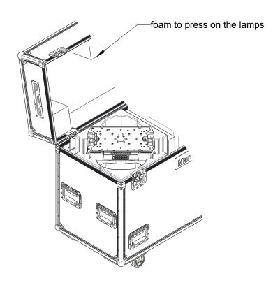
The SiP insert must be inserted into a Flightcase for 1x MAC Viper XIP: P/N MAR-91515060 2x MAC Viper XIP: P/N MAR-91515061
