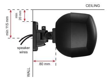
The ClickMount facilitates safe and simple installation. Note the minimum distance from the ceiling and wall as shown in the drawings.
