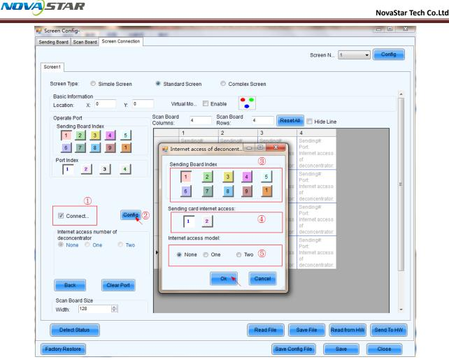
Fig. 5-17 Configuration of deconcentrator internet access
