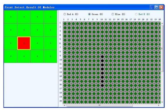
Fig. 5-77 the Error Dot Detect Result of Modules
