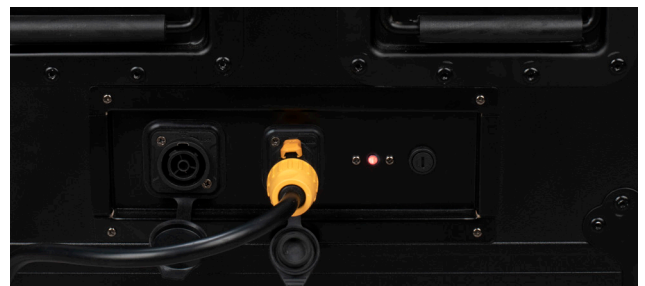
. AC Power In/Out built-in - Daisy chain power
