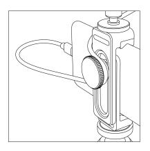
Note: Use the knob on the back of the phone clamp to keep the cable in place and out of the way of the camera.
