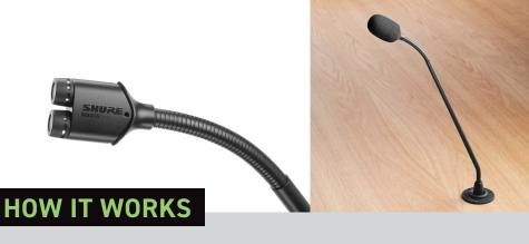
The MX415DUAL/C delivers redundant audio capture for applications that require premium results when failure isn't an option. With a unique dual capsule design, every word is captured simultaneously by two cardioid cartridges, each to a separate output preamp – providing reliable multi-feed audio for a variety of applications.
