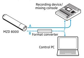
The MZD 8000 digital module receives and transmits electrical signals according to the AES 42 standard (A).
