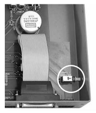
Access the internal chassis ground lift switch through a small hole in the side of the chassis.
