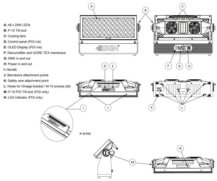
Figure 1: Parts identification and terminology
