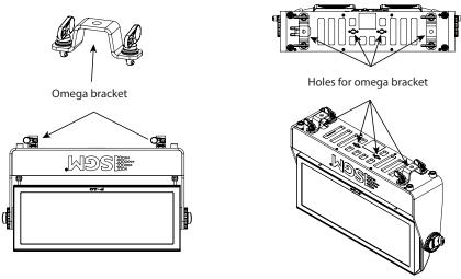
Figure 3: Base with omega bracket
