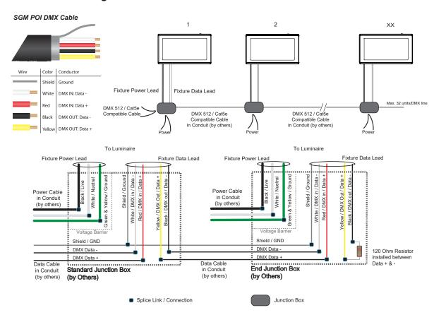
Figure 19: Connecting DMX and AC Power in P-10 POI
