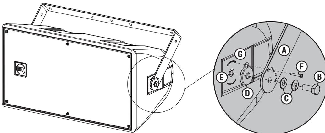
Put together the loudspeaker and the U bracket **(A)** by fastening (on both sides) a M8 bolt **(B)** into the loudspeaker hole **(E)** through the 2 washers **(C)** and the spacer **(D)**.
