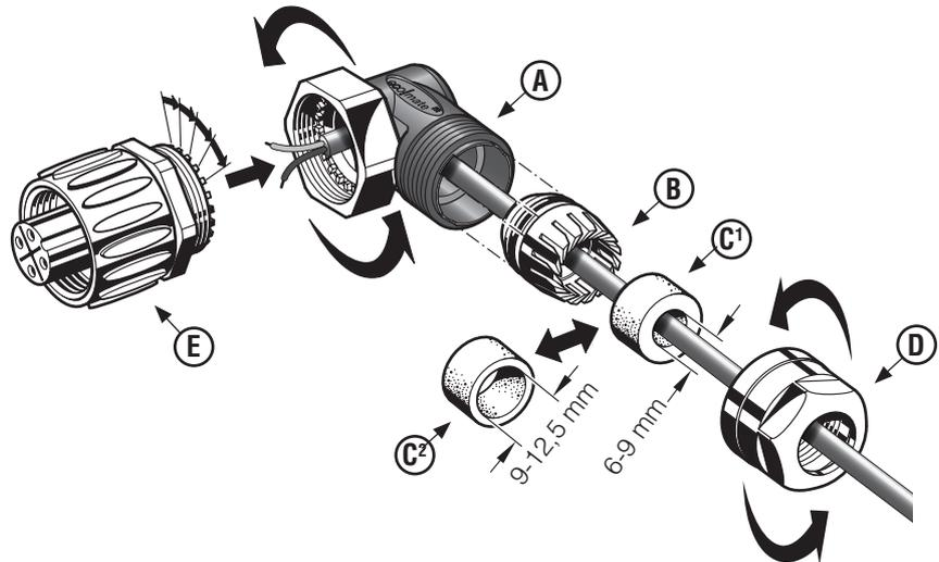
1. The **(C<sup>1</sup>)** gasket is already inserted into the clamping ring **(B)**: if necessary, replace it by the alternative one **(C<sup>2</sup>)** having a wider hole.
