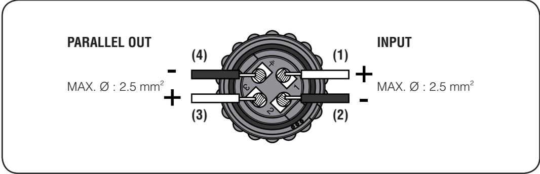
Locking at the rear side of the female contact insert (E), connect the wire coming from the amplifier output + to the contact 1 and the other wire (amplifier output - ) to the contact 2, then fix the contact insert (E) to the back shell (A).
