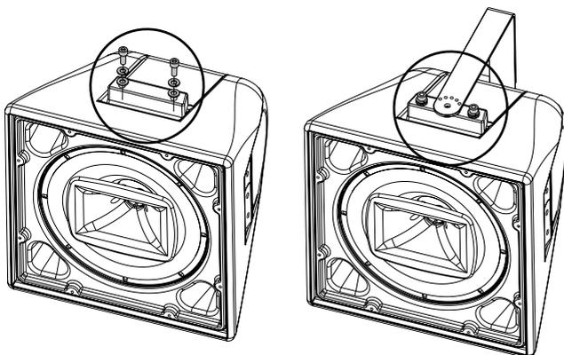
**Note:** it will be possible to remove a pair (only) of lateral bolts (used to fix the two shims) if a particular horizontal aiming angle is required”
