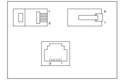
The IN port will only be used when the system has more than one PM.To interconnect two PMs, connect the OUT port of one to the IN port of the next 'in the chain' using the same wiring standard as shown in the table above. See "Systems with multiple paging microphones" on page 47 for full details.
