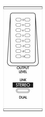
FIGURE 2 – LED Output Meter and Link Switch
