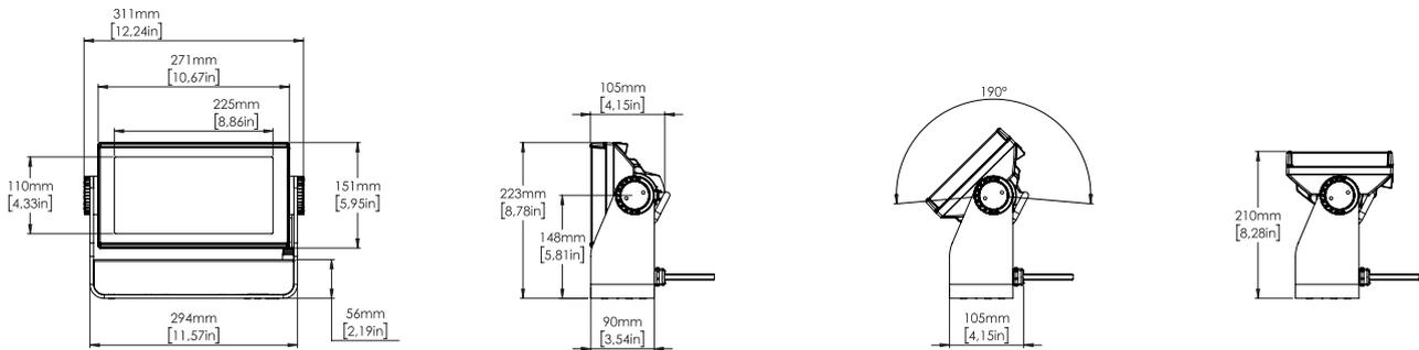
All dimensions in millimeters and inches. Drawing not to scale.
