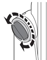
Figure 7: Q-2 Standard tilt lock
