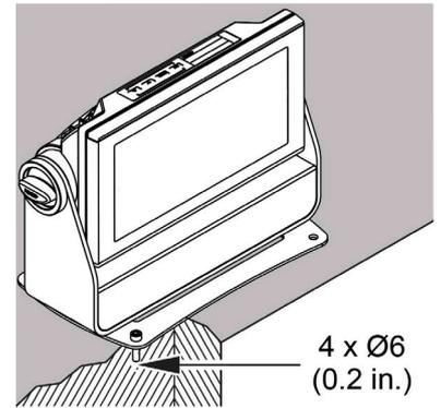
Figure 6: Q-2 mounting bracket
