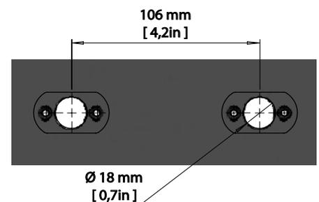
**Figure 2: Q-2 Series locking points**
