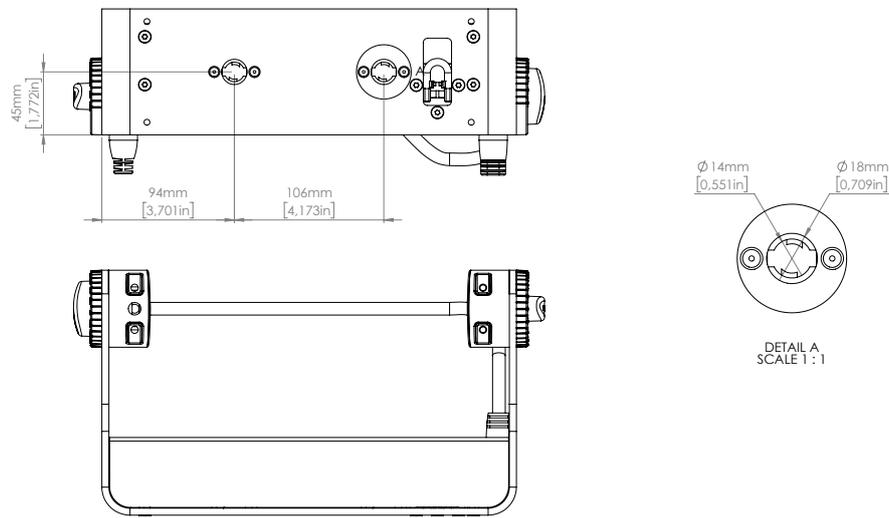
Figure 3: Dimensions for Q-2 base locking points
