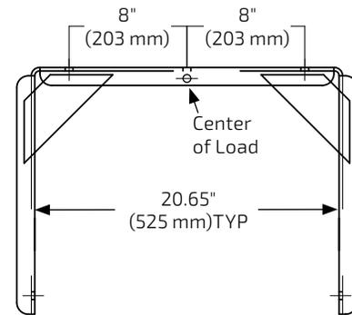
*Note: Cabinets are hand-laminated and measurements vary slightly due to the thickness of the fiberglass. Dimensions shown should not be used to fabricate hanging fixtures. Mounting points are approximate.*
