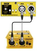
Fig.36 - Balanced XLR connections between the JX44 and SGI-44.
