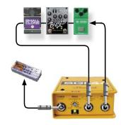
Fig.37 - Hi-Z guitar, effect and tuner connections
