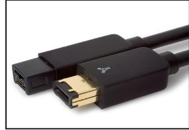
*9 pin Firewire 800 (top) to 6 pin Firewire 400 (bottom)*
