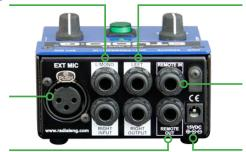
OUTPUTS - '/'' TRS connections carry program material mixed with the talkback mic output.
