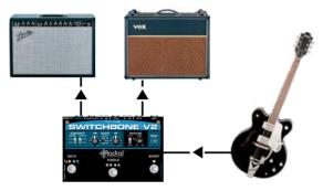
You will note that when you hit the BOTH footswitch, one of the LEDs will begin to flash. This TOGGLE mode function is designed to let you know in advance what will happen when you hit the BOTH footswitch again whereby the flashing LED will be the one that goes off. You can toggle the flashing LED by depressing the AB selector footswitch so that when you return to single amp playing, you can ensure the amp that you want on will be the one that is active.
