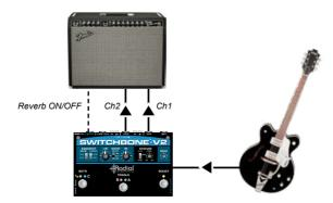
Example: When the Slingshot is set to activate on the TOGGLE it will allow you to turn on the reverb on the amp when you switch between channels.
