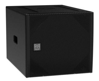
The SX115 is a versatile, passive subwoofer with an operating range of 45-100Hz + 3dB. Featuring a powerful, long excursion 15" (380mm)/4" (100mm) voice coil driver with a water-resistant cone and triple roll surround, it delivers dynamic low frequency performance from a very compact enclosure. Four reflex ports increase LF output efficiency and have a large frontal area to reduce turbulent air noise at high levels.
