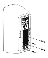
Figure 6.2: Bolt removal
