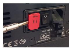
**Step 2**: Remove the fuse holder by using a flat head screwdriver as shown.
