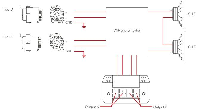
Figure 4.1: Cyclone 208i wiring diagram
