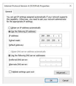
Figure 5.16: Internet Protocol Version 4 (TCP/IPv\$) properties
