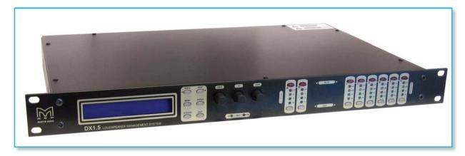
The DX1.5 is a 2 input 6 output digital loudspeaker management system for use in both live applications and fixed installations. Based on a processing platform running at 96kHz the DX1.5 offers unrivalled performance and flexibility.
