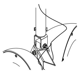
Figure 7.33: Safety wire detail
