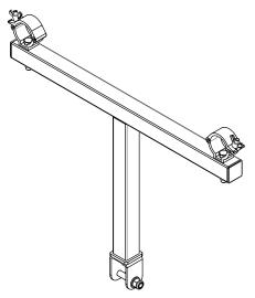
Figure 7.23: AMTB truss mount bracket
