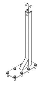
Figure 7.18: AMMB wall/ceiling bracket
