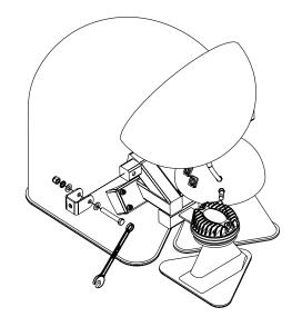
Figure 7.2: U bracket positioning
