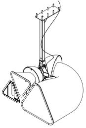
Figure 7.21: Safety wire attachment
