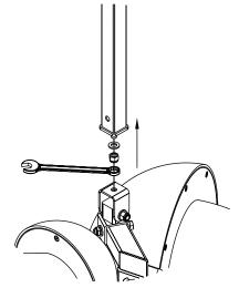
Figure 7.20: Tri motion ceiling mounting detail
