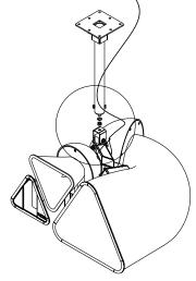
Figure 7.32: Safety wire attachment
