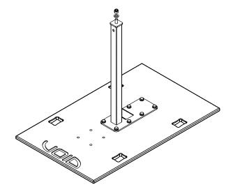
Figure 7.4: Stasys Xair/XV2 or Stasys 218 mounting board with bracket
