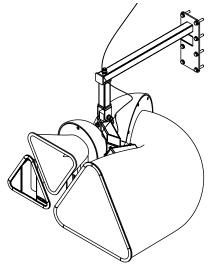
Figure 7.15: Safety wire attachment
