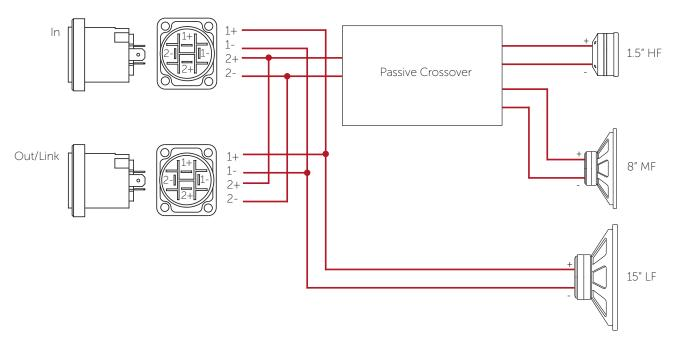
Figure 5.1: Tri Motion wiring diagram
