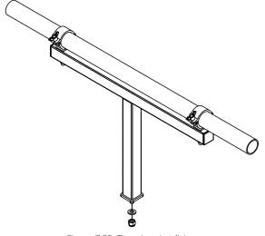
Figure 7.25: Truss bracket fixing
