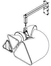
Figure 7.13: Tri Motion wall mount
