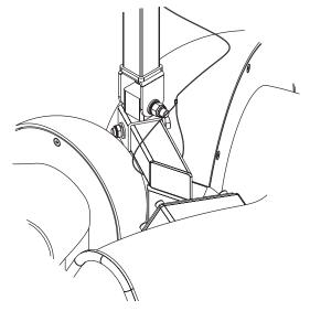
Figure 7.16: Safety wire attachment detail
