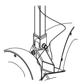
Figure 7.28: Safety wire attachment
