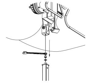
Figure 7.7: M12 Aerotight nut tightening
