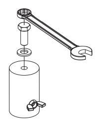
Figure 7.35: Pole mount bracket removal
