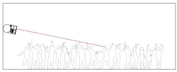
Figure 6.5: Correct loudspeaker placement
