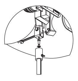
Figure 7.36: Mounting to the U bracket
