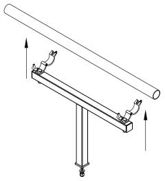
Figure 7.24: Truss bracket positioning
