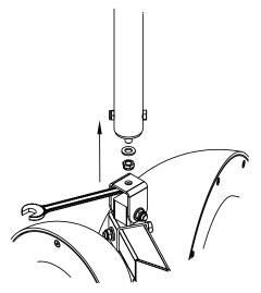
Figure 7.31: Attaching the Tri Motion
