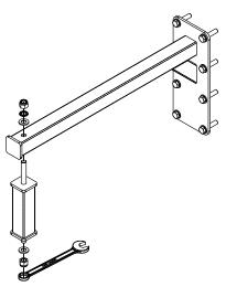
Figure 7.11: Extension piece assembly
