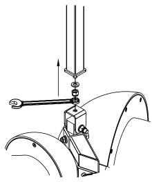
Figure 7.27: Tri Motion truss mount detail
