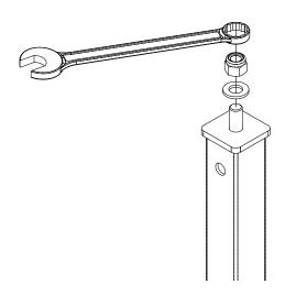
Figure 7.5: M12 Aerotight nut removal
