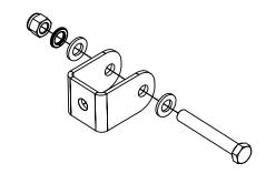
Figure 7.1: Air series U bracket
