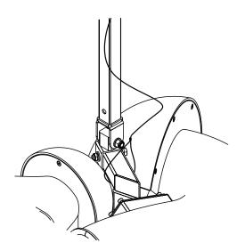
Figure 7.22: Safety wire detail
