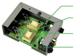
**MONO SUM -** Set and forget switch sums stereo signals to mono at both XLR outputs.
