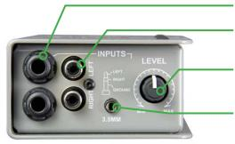
1/4" Input - Inputs can are used for stereo or two mono sources.
