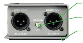
**XLR OUTPUTS** - Balanced  $600\Omega$  mic-level to drive long cables run through snakes & studio patch bays.
