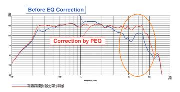
Because the TU-660 allows high range reproduction, it is possible to use EQ to raise SPL around 5–8kHz. Further, by suppressing SPL around 1–2kHz, flat characteristics can be achieved even in a horn speaker.
