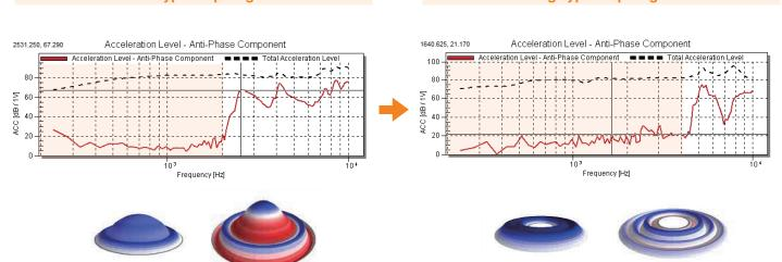
The diagram shows the differences in vibration between dome and ring diaphragms, low frequency vibration on the left, high frequency vibration on the right. Here we see reverse vibrations (red) occurring in the dome diaphragm at the higher frequency, whereas the ring diaphragm is relatively free of these and provides almost uniform vibration.
