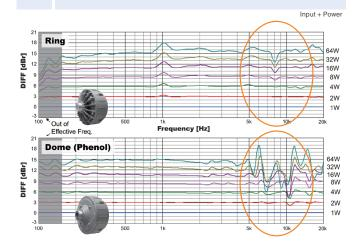
The graphs above compare the linearity of frequency characteristics against input power levels for the ring-type TU-660 construction (above) and dome-type construction of other driver units (below).
