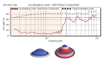
The diagram above shows a graphical representation of the state of reverse vibrations at two different frequencies. The lower frequency is on the left, the higher frequency on the right. Vibration is shown in blue, reverse vibration in red. This shows that areas of reverse vibration increase suddenly at the border of certain frequencies.
