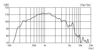
Improving these high and low range frequency characteristics is one of the issues key to improving horn speaker sound quality. Particularly, we now understand that improving the high range contributes greatly to improving the articulation of outdoor broadcasts. Attenuation in the air is more conspicuous for the high frequency ranges.
