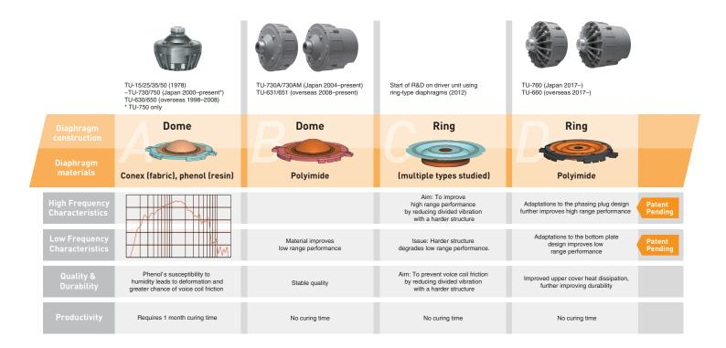
Part 01. Change materials A B C D Replacing Phenol-Impregnated Conex with Polyimide
