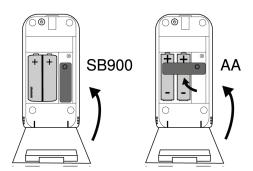
Use the small screw to the right of the batteries to secure the battery door against tampering, if necessary.
