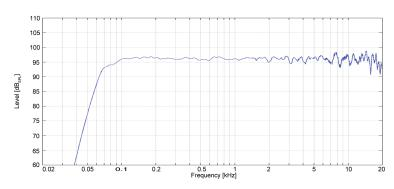
Frequency response (anechoic measurement)
