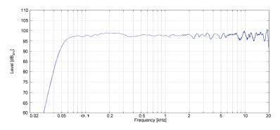
Frequency response (anechoic measurement)
