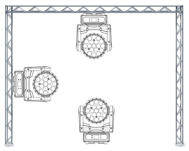
The Vizi Wash Z19 is fully operational in three different mounting positions, hanging upside-down, mounted sideways on trussing, or set on a flat level surface. Be sure this fixture is kept at least 0.2m (0.7ft) away from any flammable materials (decoration etc.). Always use and install the supplied safety cable as a safety measure to prevent accidental damage and/or injury in the event the clamp fails (see next page). Never use the carrying handles for secondary attachment.
