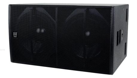
The X218 is a dual-driver, high performance subwoofer for use with BlacklineX Series full-range loudspeakers. With an operating range of 42Hz-200Hz + 3dB, it produces high output levels with low distortion and can be used singly or stacked horizontally. It features dual 18" (460mm)/4" (100mm) voice coil, long-excursion drivers in a reflex enclosure with eight large ports that reduce air turbulence at high output levels.
