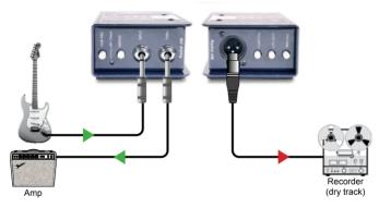
Recording a clean, dry track with a Radial direct box.
