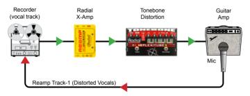
Reamping a vocal track through a Tonebone distortion pedal.
