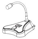
The Cloud PMI paging microphone is also compatible with the Z8MK4 and Z4MK4. It is a much simpler unit which addresses only one zone. See "Connecting a PMI paging mic" on page 14 for more information.
